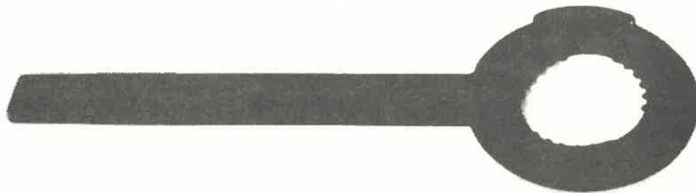
2. Five-speed flywheel holding tool (B). This tool will only be needed if you have not converted to a total loss ignition system.
